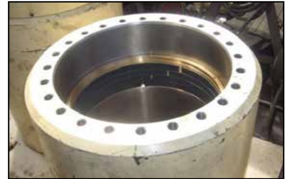
16K cut wear rings are installed in the groove.
