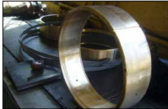
Bearing groove being machined in the old bushing.
