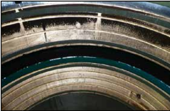
Worn, scored ram bushings (with spiral oil grooves).
